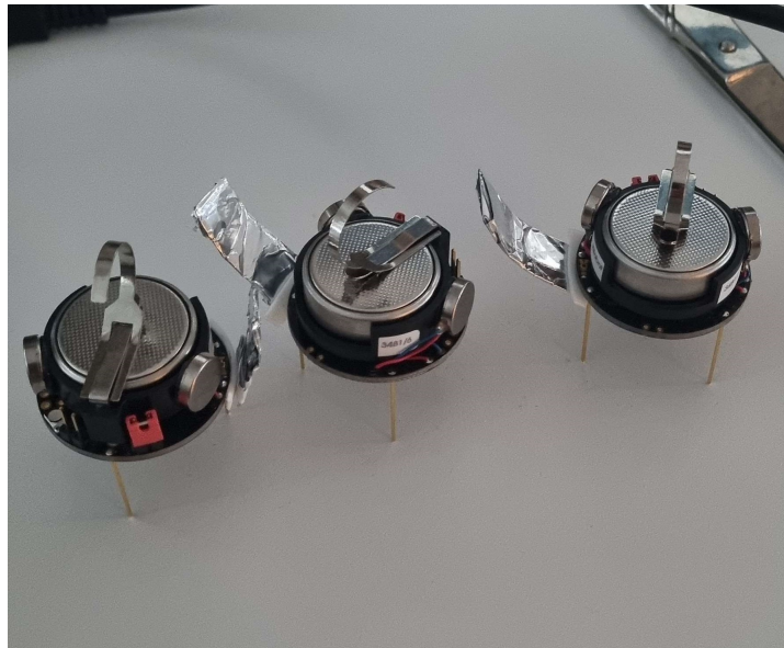
Figure 5.6: Extension of ambient light sensor built with paper wrapped in aluminum foil
