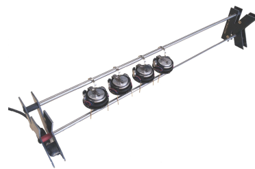
Figure 4.2: Kilobots on charger.
